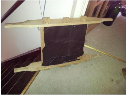
One more thing you need to do before applying the plaster. You need to drill two holes at each end of the middle spreader to take the wire that will hold on the liner. Install the wire now ready to hold on the liner.
